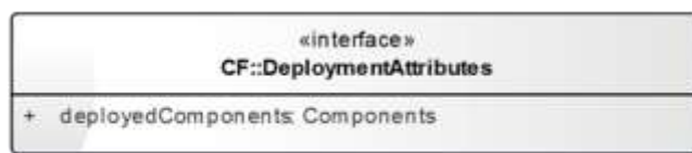
Figure 3-19: DeploymentAttributes Interface UML
