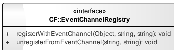
Figure 3-25: EventChannelRegistry Interface UML
