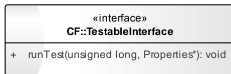
Figure 3-9: TestableInterface Interface UML
