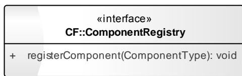
Figure 3-23: ComponentRegistry Interface UML
