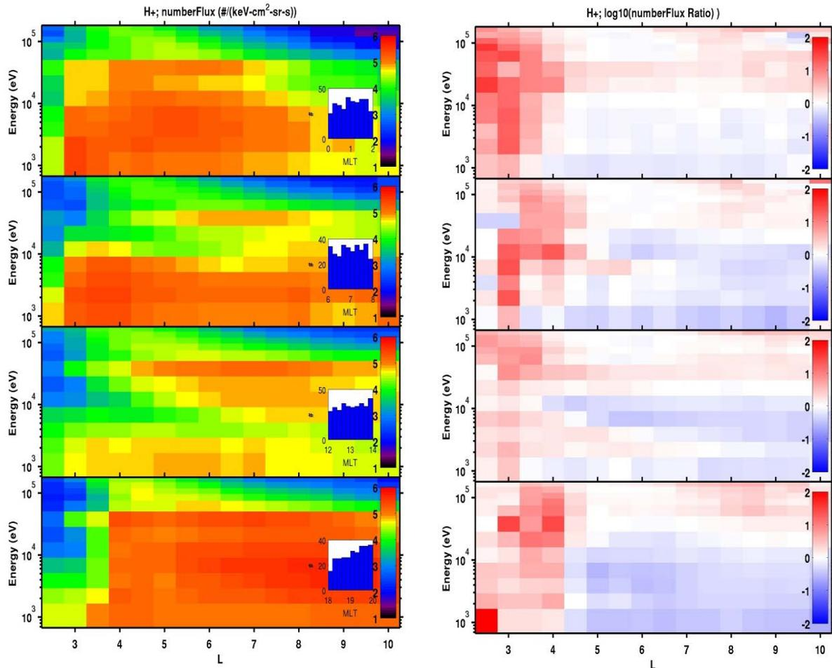
**Figure 77. Energy- $L$  spectrograms at four different local times (left) and their flux ratios with the *Roeder et al.* [2005] database (right).**
