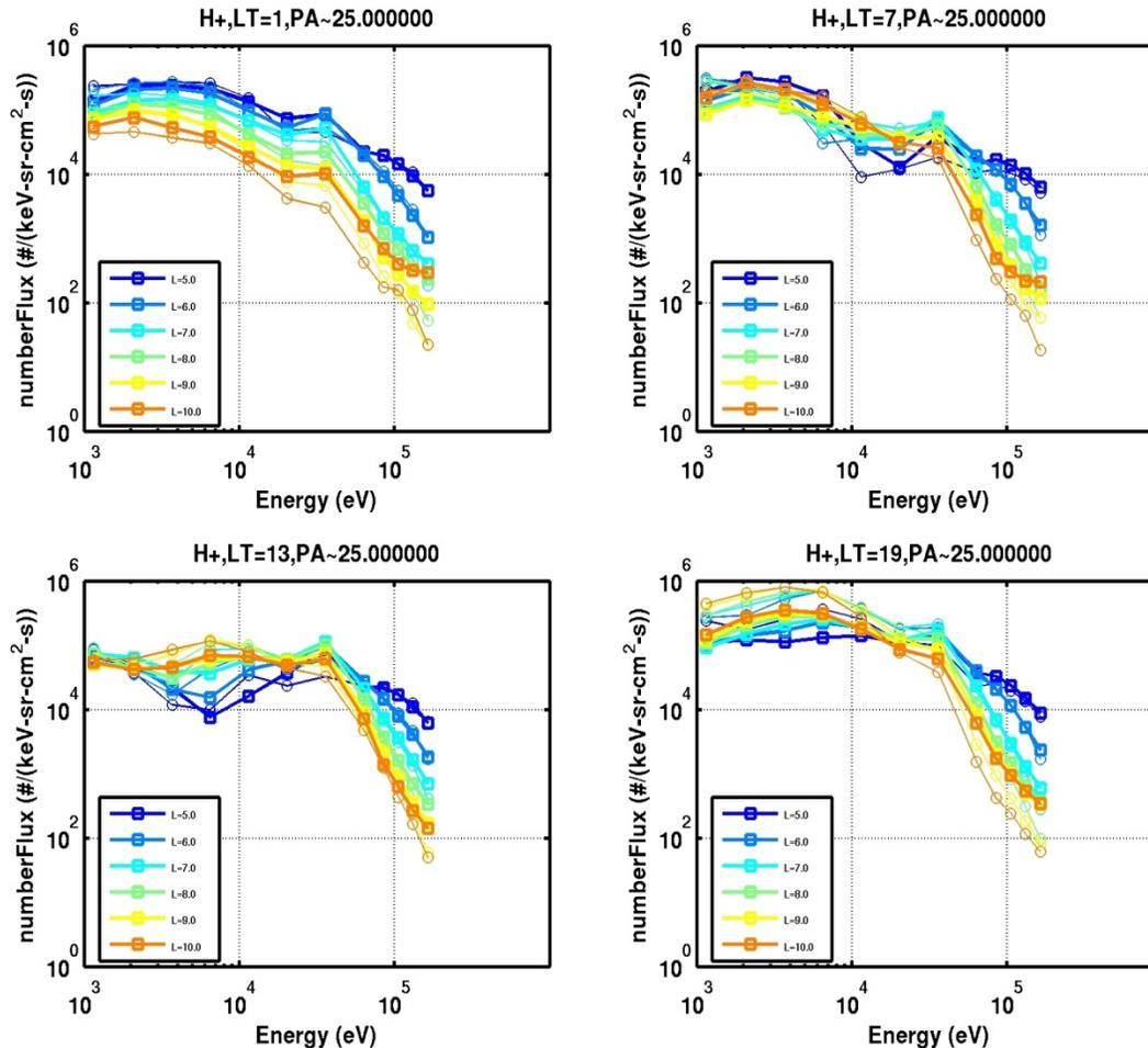
**Figure 76.** Spectra at an equatorial pitch angle of  $25^\circ$  and four different local times near midnight (top left), dawn (top right), noon (bottom left), and dusk (bottom right). In each panel spectra are colored by  $L$  value, thin lines are taken from the *Roeder et al.* [2005] database, and thick lines are aggregated in our analysis.
