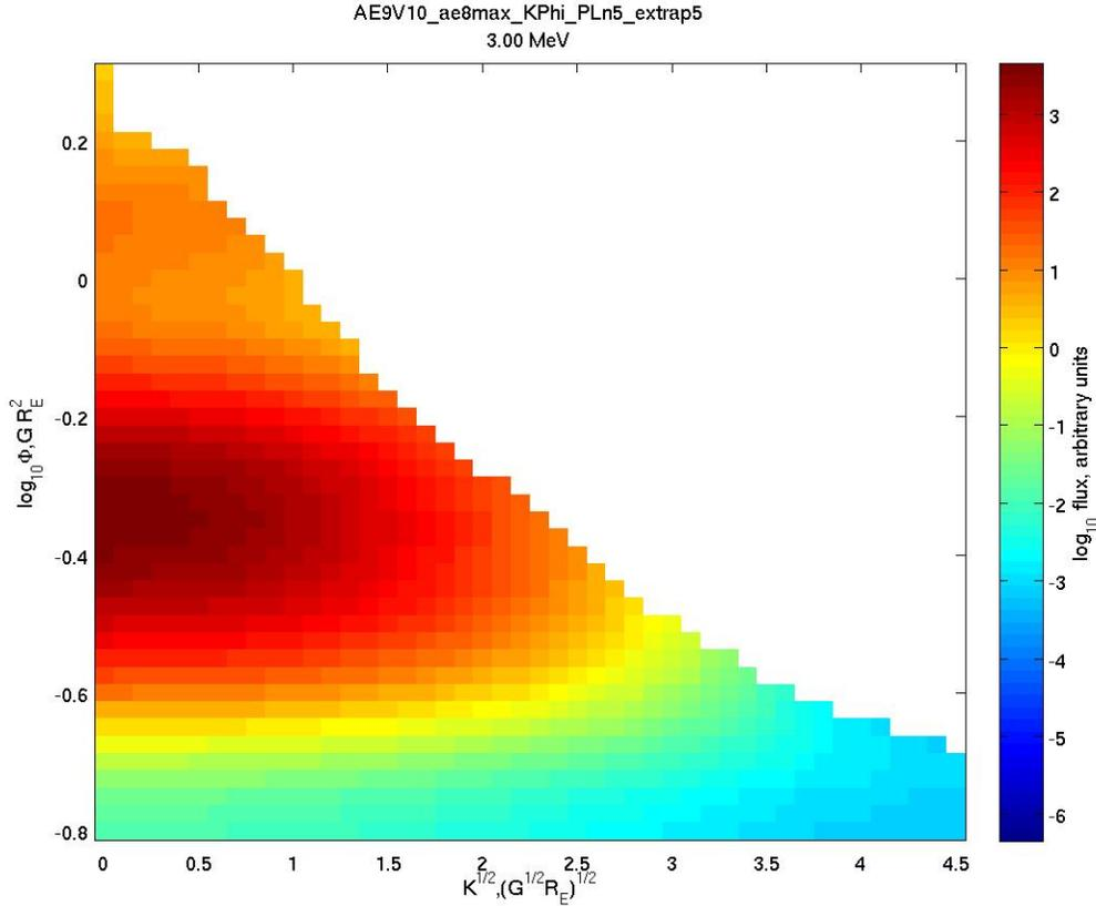
Figure 19. An AE9 V1.0  $K$ - $\Phi$  template at 3 MeV derived from AE8-MAX. The orange region at top left is the inner zone, and the dark red region is the outer zone.
