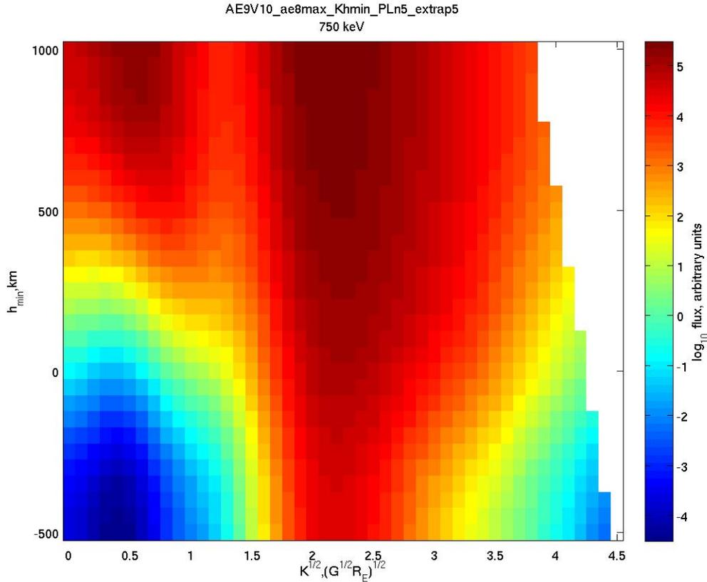
**Figure 18.** An AE9 V1.0  $K$ - $h_{min}$  template at 750 keV derived from AE8-MAX. The deep red region at top left is the inner zone, and the deep vertical red region in the middle is the outer zone. The atmospheric loss cone is at  $h_{min} = 100$  km, so this template implies significant quasi-trapped flux ( $h_{min} < 0$ ).
