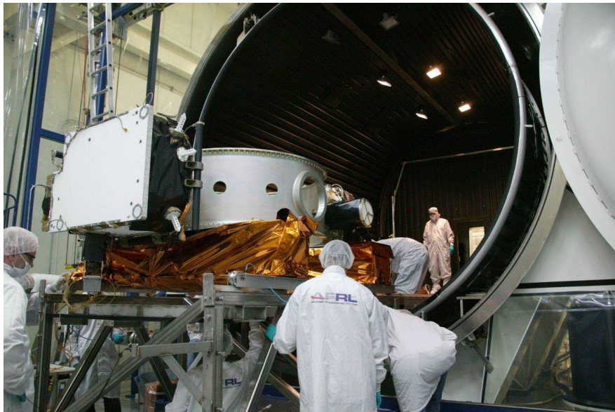
DSX environmental testing at in-house facility
